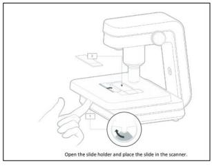
To insert our slide, we need to feel under the open slide tray for a switch that will open and close the tab that secures our slides.
