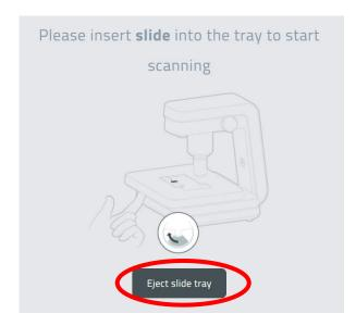
Click on the "Microscope" Tab on Left top corner. Click on "Eject slide tray" to insert our slide.
