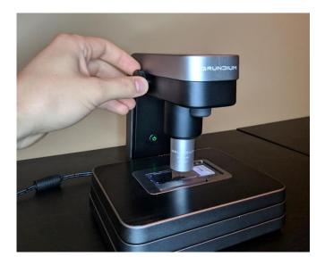
Move to sample using "Navigator" view to monitor coarse focus, When the microscope says, "focus in range", click the "AF" (auto focus) button in the bottom right corner of the live view window.
