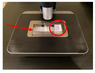
Open this tab, insert the slide with the label to the right (label should be in the more open end) and close the tab again to secure it in place
