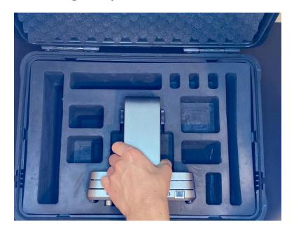
On the bottom of the scanner there is a transportation pin that prevents the slide deck from moving in the carrying case. This needs to be removed before use, by turning it counterclockwise. The pin can then be returned to the carrying case.
