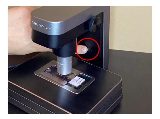
To turn on our microscope, press the power button at the front of the scanner neck. The button should start blinking red, then turn solid green. This means that the scanner has powered on and is connected to the internet.
