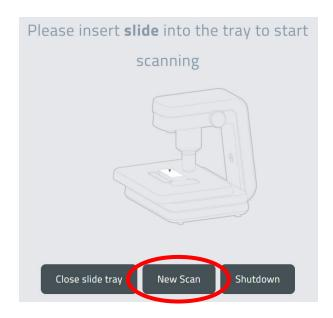
Click on "New Scan" to start scanning. On Microscope, there will be two lights, a red and a blue flashing one, which is the microscope taking a birds eye view of the slide, and a short white burst which is a photo of the label (on the right side).
